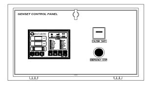
Datakom DKG307 digital automatic control module Hourmeter
