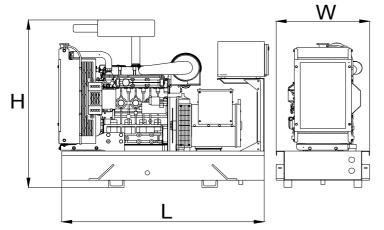
Length, L 1,4 m Heigth, H 1,2 m Width, W 0,7 m Weight, Total 550 kg
