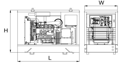
Length, L 1,5 m Heigth, H 1,25 m Width, W 0,8 m Weight, Total 700 kg
