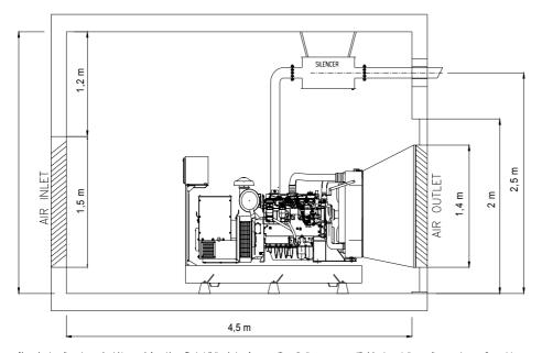
Adove drawings amensions and weights are only for guidence. For installation design of your specific application, necessary certified drawings, at site consultancy service as well as maintenance and installations manuals will be provided by Cukurova without any charge without notice.
