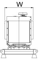
Length, L 2,6 m Heigth, H 1,5 m Width, W 0,9 m Weight, Total 1600 kg
