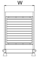
Length, L 3,3 m Heigth, H 2 m Width, W 1,2 m Weight, Total 2100 kg
