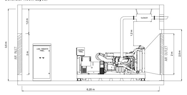
Above drawings dimensions and weights are only for guidence. For installation design of your specific application, necessary certified drawings, at site consultancy service as well as maintenance and installations manuals will be provided by Cukurova without any charge
