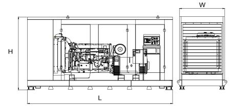
Length, L 4,5 m Heigth, H 2,5 m Width, W 1,4 m Weight, Total 4600 kg
