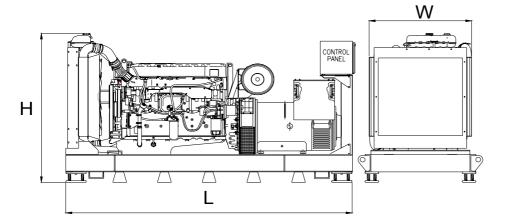
Length, L 3,1 m Heigth, H 1,7 m Width, W 1,1 m Weight, Total 3400 kg
