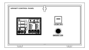
Datakom DKG307 digital automatic control module Hourmeter
